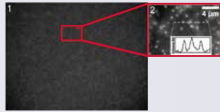
1) Fluorescence image of the beads near the surface of the hydrogel. 2) Intensity profile of the fluorescent beads.
