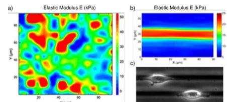
*Our tissues are 1 million times softer than the plastic of culture dishes: here, human pituitary gland demonstrates rigidities around order of kPa, with micron-scaled heterogeneities.*
